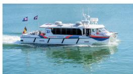
**Hydrogen dual fuel combustion, passenger vessel, size 14m\*4.2m**
