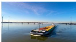
**Battery/diesel – electric powertrain, containervessel, size: 110m\*11.45m**
